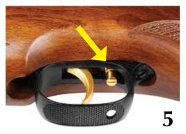
There's a large adjustment screw located behind the trigger blade (Fig. 5). This screw is accessible through the hole on the bottom of the triggerguard. Turning it clockwise increases trigger-pull; counterclockwise decreases the trigger-pull. Improper adjustments may make the airgun unsafe.
