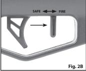
**AWARNING:** KEEP THE AIRBOW IN THE "ON SAFE" POSITION UNTIL YOU ARE ACTUALLY READY TO SHOOT. THEN PUSH THE SAFETY LEVER TO THE "OFF SAFE" POSITION.
