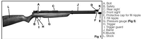
Your new airgun is unique because it operates on either compressed air or  $CO_2$ , To fill and shoot with  $CO_2$ , an optional  $CO_2$  fill adapter must be purchased. This owner's manual describes operating the gun with compressed air only. The manual that comes with Crosman's  $CO_2$  adapter describes operation on  $CO_2$ .
