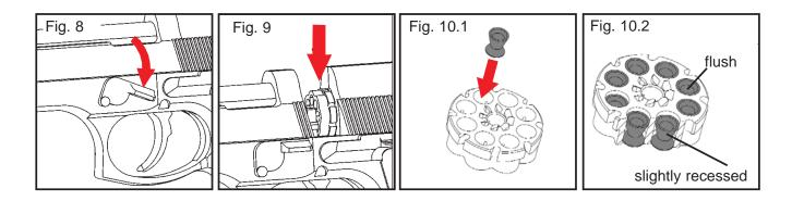
Remove the pellet clip and load the pellets head first (see Fig. 10) into the clip insuring that each pellet is completely inserted.
