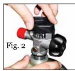
Tighten valve by hand. Make sure the metal of the tank touches the metal of the valve. (Fig. 3)
