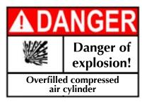
Do NOT exceed <u>maximum fill</u> <u>pressure</u> of 310 bar/4,500 psi at room temperature!
