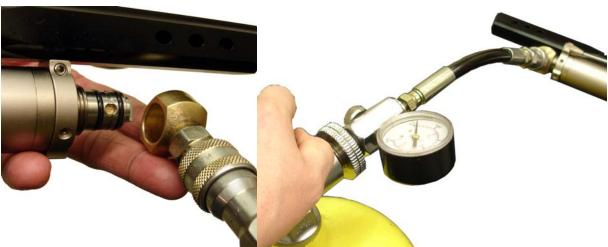
Once the connector is exposed the female part of the filling kit can be place on the male and press all the way on making sure that the 'O' rings on the male part are covered.
