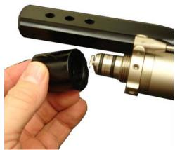
Removing the end cap is achieved by unscrewing in an anticlockwise direction.
