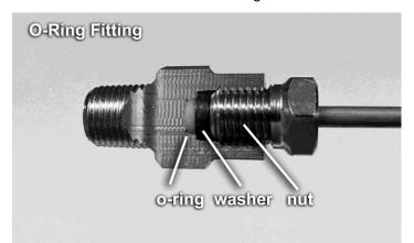
used for the lower piston. The nut no longer contributes to the sealing so do not over tighten.
