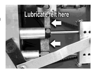
Your Shoebox is equipped with wicking felt oiler strips. A felt strip is pinched in the black nuts at the ends of each cylinder. **USE ONLY SILICONE OIL** that is supplied with your unit to saturate the felt strips. The oil will wick onto the pistons as it runs. After about 10 hours check the felt strips and if needed, apply more silicone oil.
