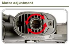
The motor adjustable screw is at the bottom of the grip. Use a screwdriver to adjust.
