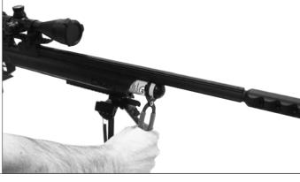
Screw 88 g  $CO_2$  cartridge into stock, narrow end first.
