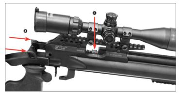
Place a pellet in the breech. Observe correct position! O Push the cocking lever forward until it clicks into place.
