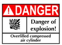
Do NOT exceed <u>maximum fill pressure</u> of <u>200 bar</u> at room temperature!
