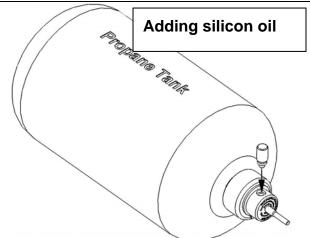
Take off Parts #8 (Silicon oil adapter) and drop some silicon oil in order to lubricate your GBB Airsoft. Then, put part #8 back to XG02. (Propane gas is dry and doesn't come with oil.)NOTE: \* If there is propane leaking when you take off #8 silicon oil adapter, please uninstall XG02 immediately. You either don't install XG02 correctly or your XG-02 is not working functionally. \*\* When you put part#8 back to XG02, please remember the oring (parts #10) is still there.
