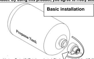
Smoothly turn Parts #6 (Rotating adapter) Clockwise to install the XG-02 adapter. Do NOT cross the adapter threads! If there is any leaking after you install the XG-02, please take XG-02 out of propane immediately. Leaking only happens when you didn't install correctly. (\* How to tell it is leaking? You can hear the leaking sound and you can smell the propane odd odor.) (\*\* When you take off XG02 from Propane tank, remember to hold tight of both XG02 and tank.)
