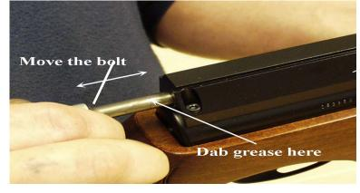
Apply a small dab of grease on the loading bolt and work-in by moving the bolt forwards and backwards. Wipe off excessive grease. Preferred grease is 'napier g95 gun grease'
