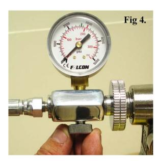
6. Disconnect the charging kit from the rifle and turn the knurled bezel until the hole in the air reservoir tube is closed. This will prevent any dust or dirt from contaminating the air reservoir and valves.
