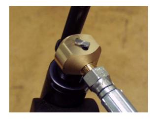
It is a wise precaution to hold the female part of the connector, during the filling procedure, as shown in the pictures below. This will ensure the female adaptor is located completely over the male part and prevent any accidental dislodging of the connector before you start to refill the cylinder.
