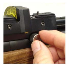
On the left side of the rifle is an indicator to help select your power setting. + = High, - = Low. The marks do not indicate a particular power as this would change depending on the pellets used.
