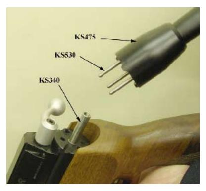
Part no. KS340 has to line up with the hole in the center of the cover on the front end of the stock piece (KS475), a small amount of pressure can then be applied to the rear stock so that the three locating pins (KS530) push through the corresponding holes in the striker body.
