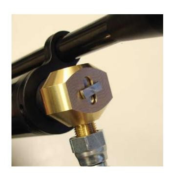
If the rifle is empty the mechanism will need to be cocked to allow the firing valve to close. If the rifle is not cocked when the bottle is opened or the pump used, the air will past the valve and exhaust through the barrel.
