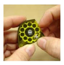
Be very careful not to damage the indexing spring when demounting or mounting the magazine. Follow the instructions carefully.
