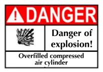
Do NOT exceed <u>maximum fill pressure</u> of <u>206 bar/3000 psi</u> at room temperature!
