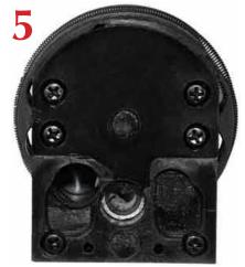
Image 5: After seating pellet, turn mag so pellet appears in center hole and left hole is ready to accept another pellet. Repeat steps 1-5 until mag is filled.
