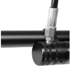
When you reach 2900 psi, turn off the valve from your fill device and exhaust the moisture and air from the hose. Remove the hose and probe from the gun.
