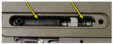
Using a high-quality gun lube (do not use household oil such as WD-40 or silicone), put 2-5 drops on the two bolt sections shown above. Drop the lube along both sections. Replace the transparent faceplate.
