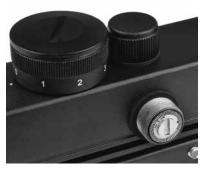
Once the protective black caps have been removed, you can adjust the elevation and windage. Insert either a coin or small flat-bladed screwdriver into the slot on top of the knob and turn. You will hear and feel noticeable clicks to make it easier to adjust and readjust your dot sight.
