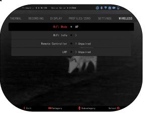
Press and hold for 2 seconds the Up Button and the OK Button to Pair the X-TRAC 5 to your ATN compatible device.
