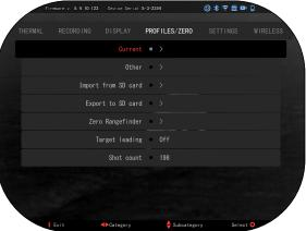
Open the Shortcut Carousel and navigate to the Wrench Icon. Scroll to Profile/Zero and then Select Current. Use the Down Button to navigate to RAV calibration. Press the Right Button to enter RAV calibration. You should see a velocity rating in the upper left corner (
