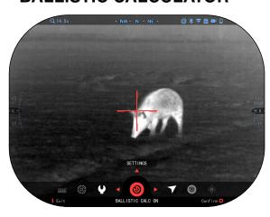
The ThOR 5 has a fully integrated Ballistics Calculator that enables your scope to seamlessly adjust its point of impact. The first step in utilizing this function requires you to enter all relevant information into the Profile that is being used.
