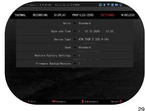
DEVICE TYPE — to make all features work correctly you need to choose the type of lens you have. (Example: 3x stands for 3-12 and 5x stands for 5-20).
