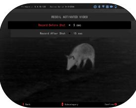
When a shot is fired and your scope experiences recoil (some airguns may not provide enough recoil for RAV to be activated). The scope will record video prior to the shot being taken, the moment of, and some time after. Exact settings may be adjusted in the System Settings.
