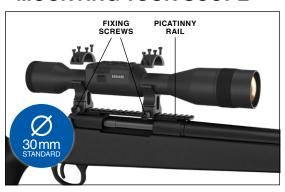
The ThOR 5 has a 3.5-inch eye relief (90 mm), and can be mounted using 30 mm mounting rings. ATN has provided two standard rings and one L shape ring. The L shape ring is for those instances when you need extra eye relief for certain rifles. First, choose your preference of rings and position and mount the bottom portions of your rings to your rail for optimal eye relief. Place
