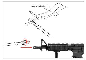
Put the safety ON SAFE and remove the magazine. Prepare a thin rod with a length of approx. 16 inches. Attach a piece of cotton fabric to its end and clean the barrel with some silicone oil. The exposed metal parts should be wiped clean using a slightly oiled cloth after handling to prevent rust. Use light acid free and resin free oil. RWS Spring Cylinder Oil is excellent for this.
