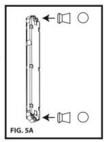
BBs) toward you, insert any .117 caliber (4.5mm) pellet or BB into each of the visible ammo clip openings at each end of the magazine. (FIG. 5A). Daisy brand BBs and Pellets are recommended.
