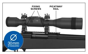
rail for optimal eye relief. Place the scope on the bottom half of the rings you just mounted, verifying you have sufficient eye relief for your platform. Place the top portion of your ring over the mounted bottom portion, make sure the holes align and the screws turn easily. Apply equal torque to all screws with the provided Allen wrench. Make sure your rings are tight on your rifles rail and will not come loose due to recoil.
