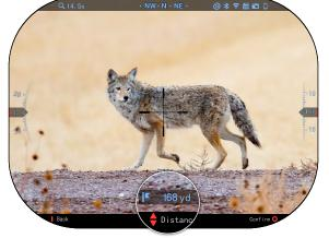
Change distance value using the Keypad buttons. To accept the new distance, press the OK button.
