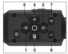
To TURN ON the device, press and hold the POWER button until you see the ATN splash screen.
