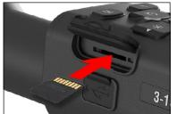
The device is equipped with a microSD Card and USB (type C) ports. You can find them under the rubber caps on the right side of the device (we marked the caps with appropriate icons).
